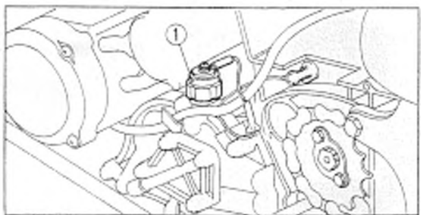
Fig. 5-43 ① Oil pressure control switch
