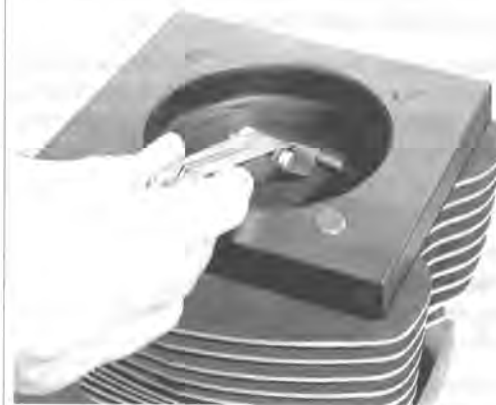
Figure 3-62. Measuring Ring Gap
