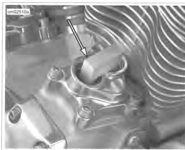
Figure 3-86. SCREAMIN' EAGLE Magnetic Lifter Holder
