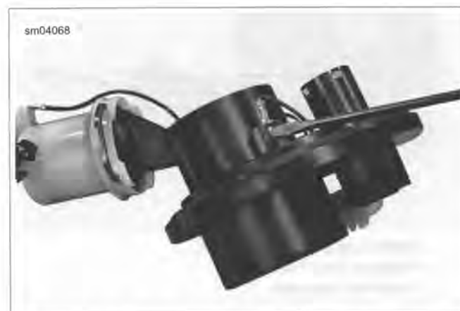
Figure 4-14. Remove Ground Wire Spade Terminal From Top Plate
