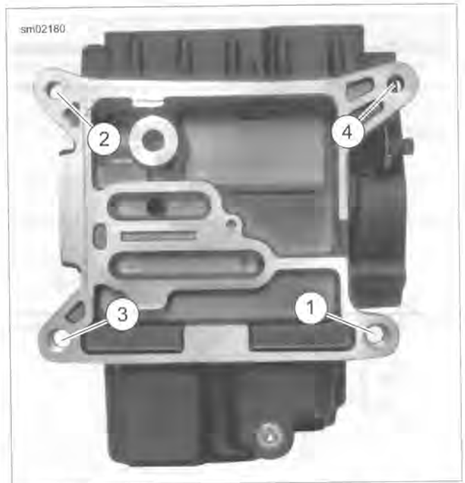
Figure 6-57. Transmission Housing to Crankcase Torque Sequence
