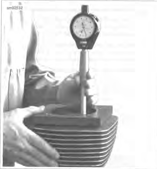
Figure 3-57. Measure for Out-of-Round and Taper
