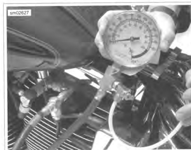
Figure 4-3. Fuel Pressure Gauge Installed (Typical)
