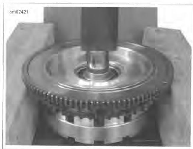
Figure 5-32. Pressing Clutch Hub From Bearing
