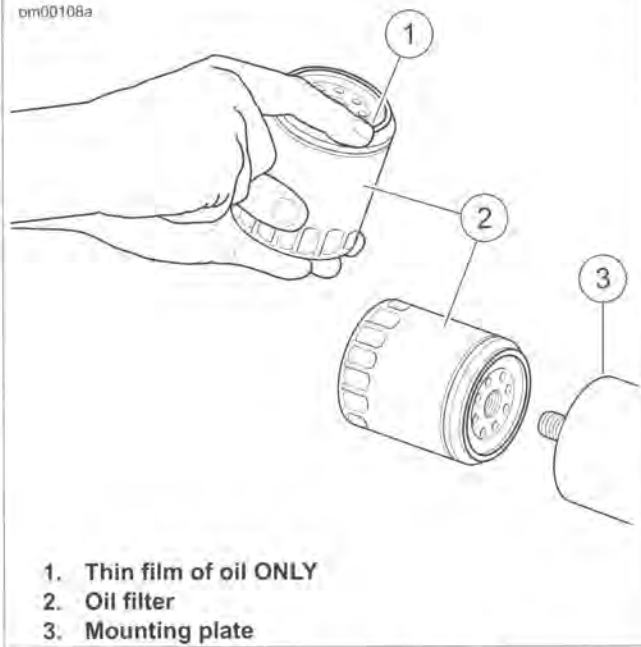
Figure 1-4. Applying Thin Oil Film
