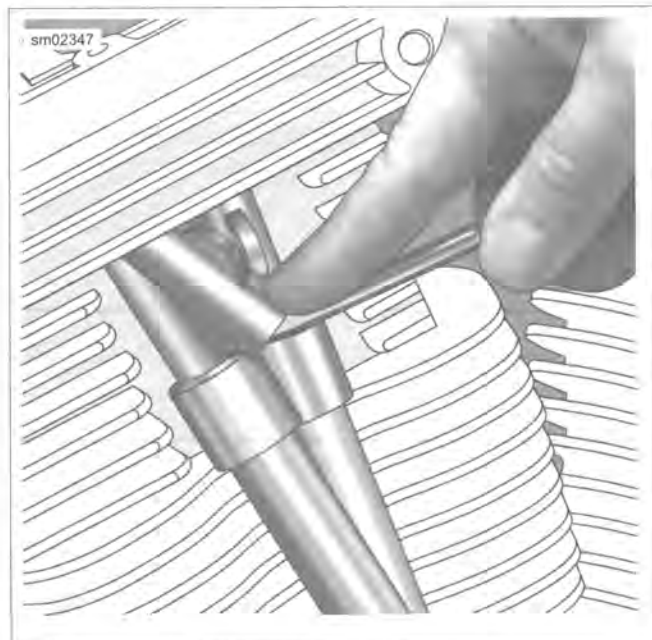
Figure 3-83. Install Spring Cap Retainers
