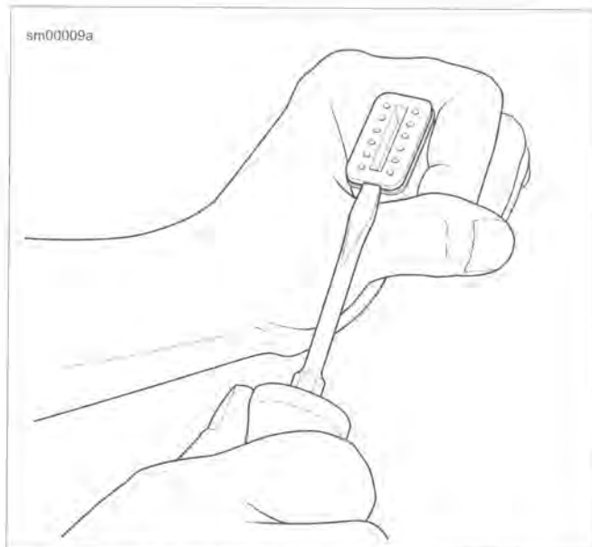
Figure A-31. Deutsch DT Sealed Connector: Remove Secondary Locking Wedge
