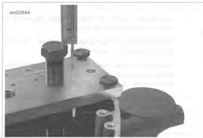
Figure 3-105. Measure from Top of Forcing Screw to Support Plate
