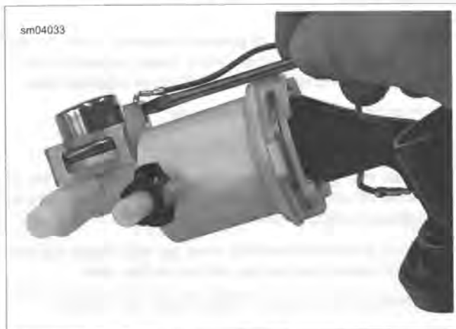
Figure 4-17. Remove Ground Wire Spade Terminal From Fuel Filter Shell
