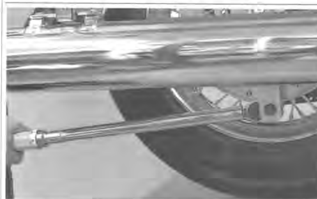
Figure 1-27. Install Tool Perpendicular to Torque Wrench
