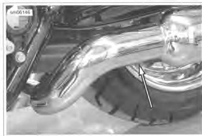
Figure 4-42. Crossover Pipe Heat Shield
