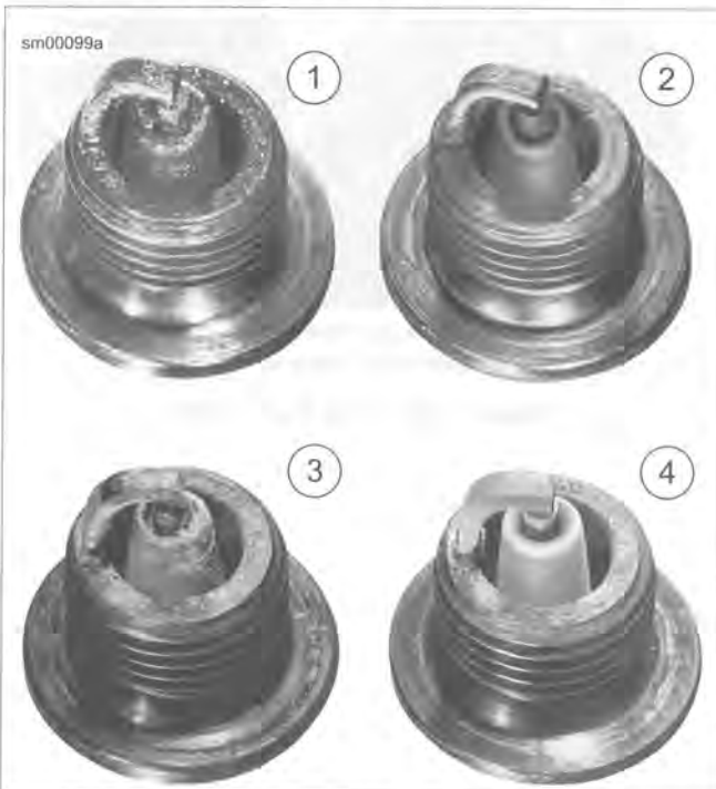
Figure 1-36. Spark Plug Deposits
