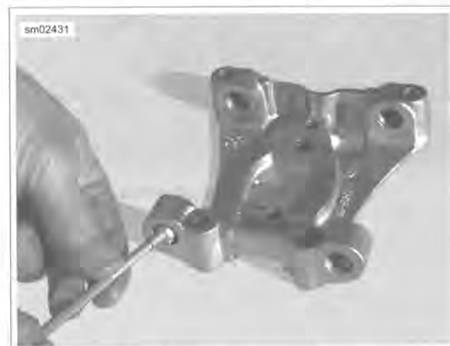
Figure 3-28. Checking Support Plate Bore
