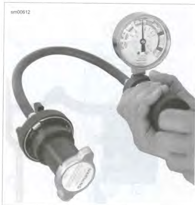
Figure C-2. Pressure Cap Test
