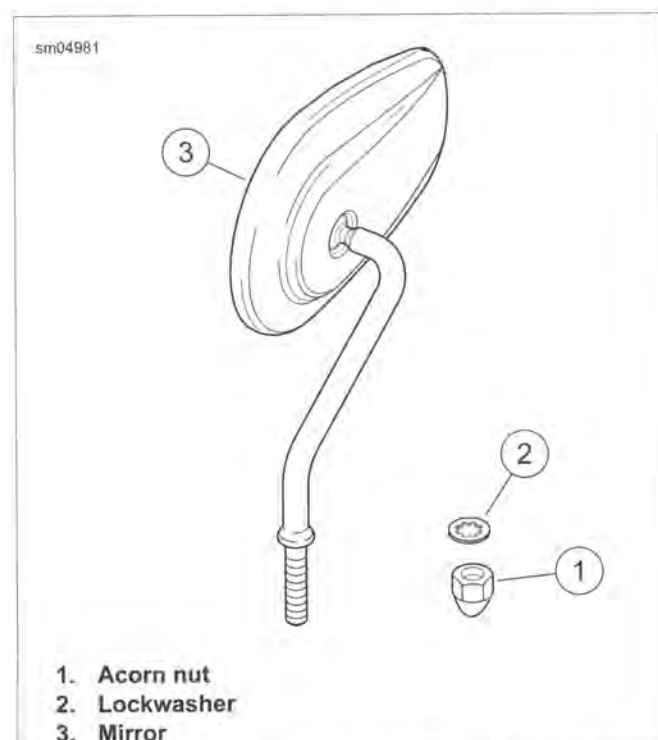
Figure 2-107. Mirror Assembly (All Models Except FLHX/S)
