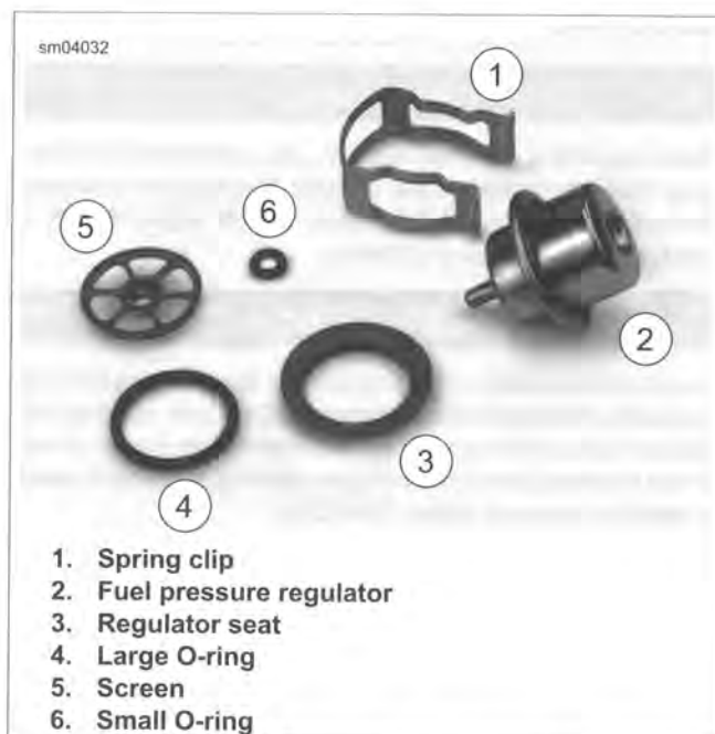
Figure 4-20. Fuel Pressure Regulator Assembly
