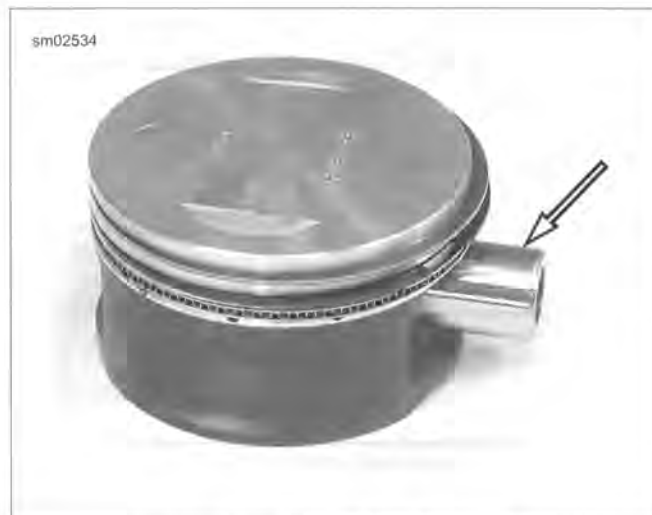
Figure 3-59. Piston Pin Clearance
