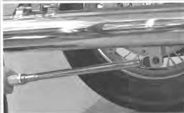
Figure 2-7. Install Tool Perpendicular to Torque Wrench
