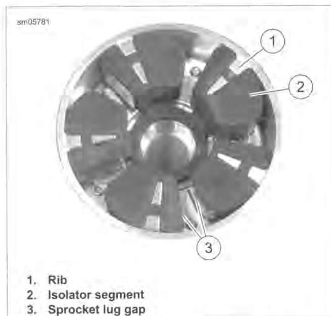
Figure 2-9. Install Isolator in Wheel
