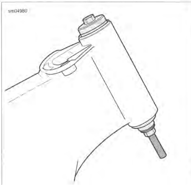
Figure 2-70. Install Steering Head Bearing Cups
