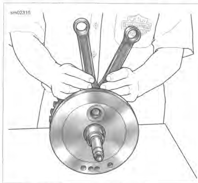
Figure 3-135. Connecting Rod Bearing Clearance
