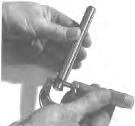
Figure 3-29. Checking Shaft to Support Plate Fit
