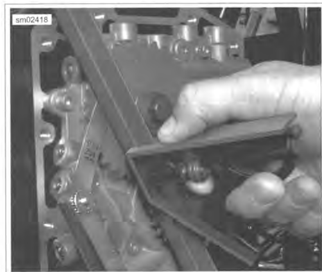
Figure 3-110. Check Alignment of Crank and Rear Cam Sprocket Faces
