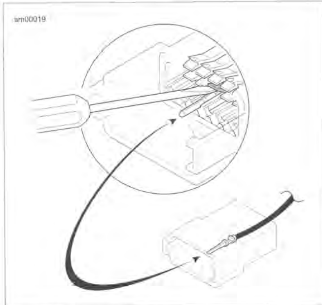
Figure A-34. Deutsch DT Sealed Connector: Press Terminal Latch and Back Out Pin
