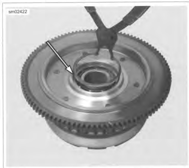
Figure 5-33. Install Clutch Shell Retaining Ring with Flat Side Against Bearing
