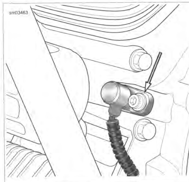
Figure 7-53. Remove CKP Sensor Mount Screw
