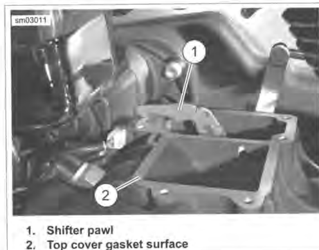
Figure 6-10. Set Shifter Pawl on Gasket
