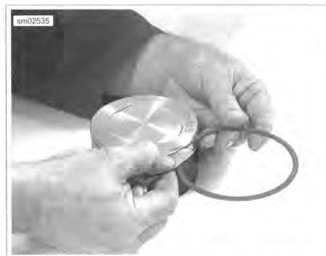
Figure 3-60. Measure Piston Ring Side Clearance
