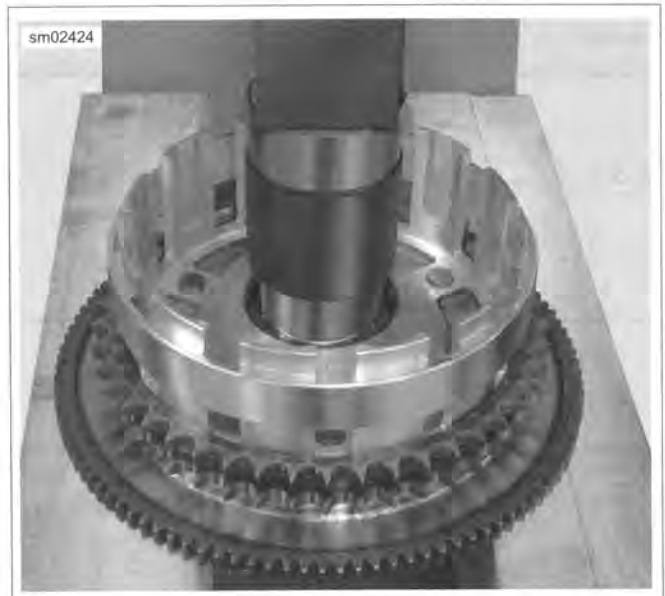
Figure 5-34. Pressing Bearing From Clutch Shell
