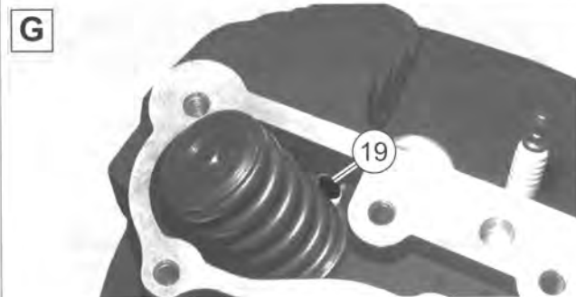
Figure 3-2. Engine Oil Flow: Top End
