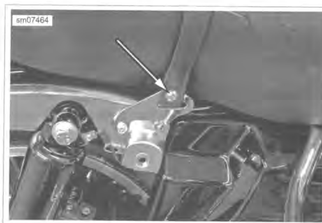
Figure 2-110. Seat Strap Screw
