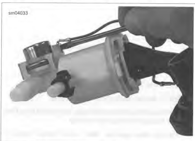
Figure 4-19. Remove Ground Wire Spade Terminal From Fuel Filter Shell
