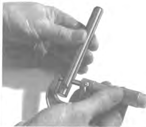
Figure 3-31. Checking Shaft to Bushing Fit
