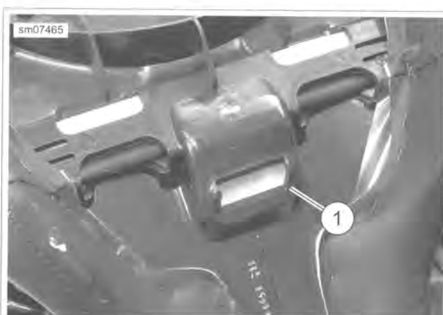
Figure 2-110. Seat Strap Screw
