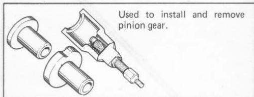
Part No. 96830-51 Pinion Gear Puller and Collars
