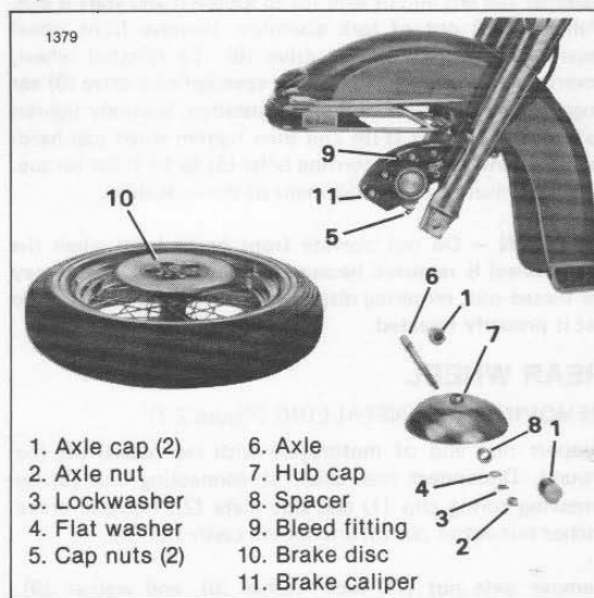
Figure 2-5. Front Wheel Removal — FL
