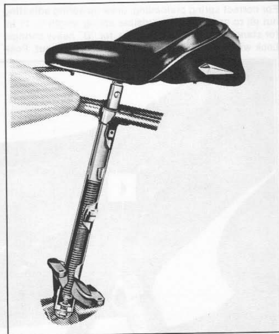
Figure 2-47. Cutaway of Seat Post Springing
