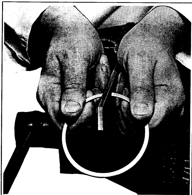
Figure 3C-8. Filing Ring Gap
