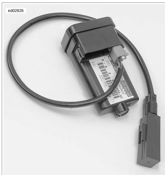
Figure 3-1. HFSM and Antenna
