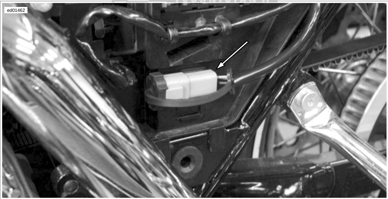
Figure 4-86. ECM Data Link Connector
