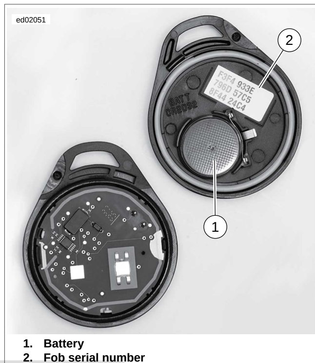
Figure 3-17. Open Fob: HFSM
