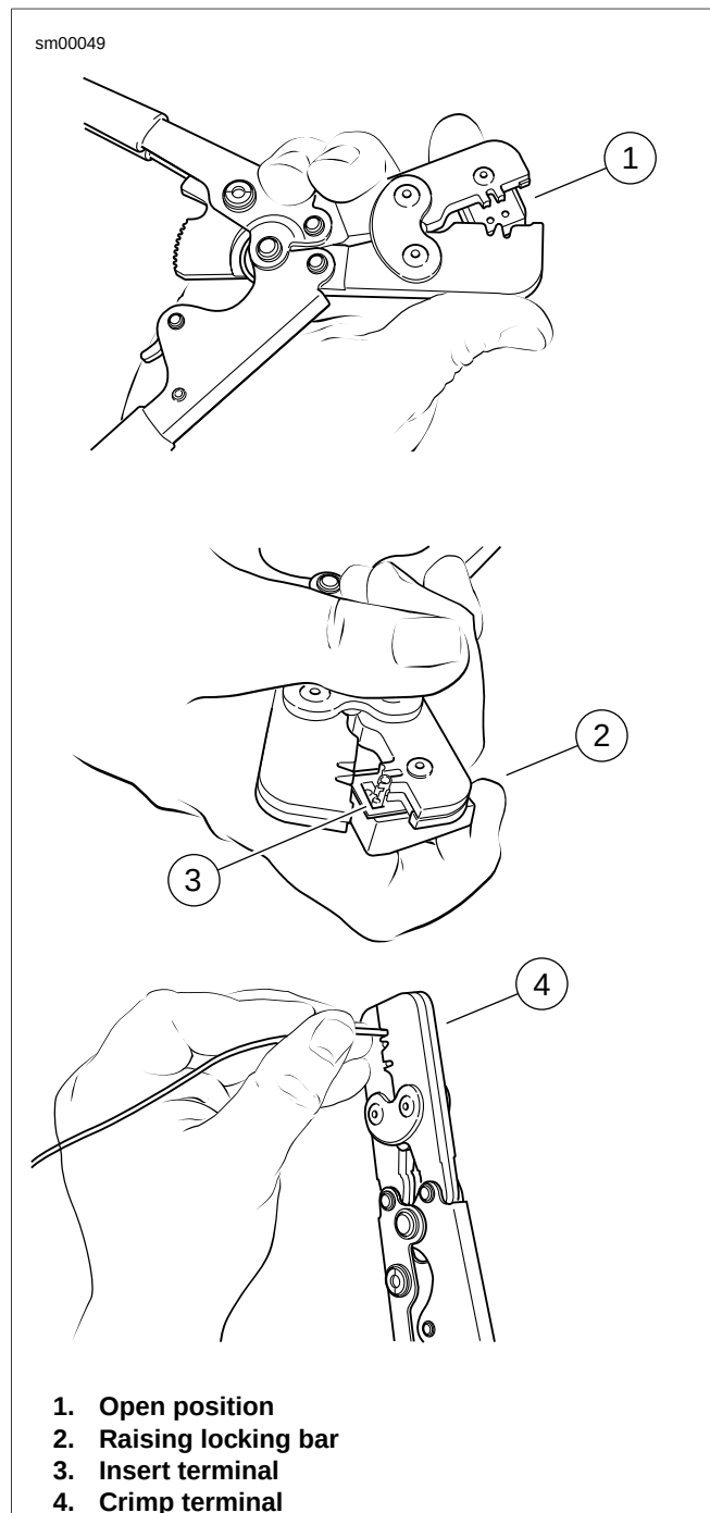
Figure A-47. Packard Micro 64 Connector: Terminal in Crimper
